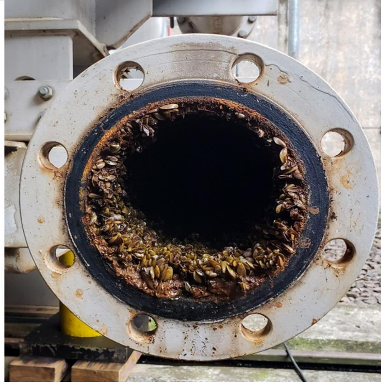
Golden Mussels colonizing a water pipe at a hydroelectric plant in Brazil ( Mountinho, 2021 ).
