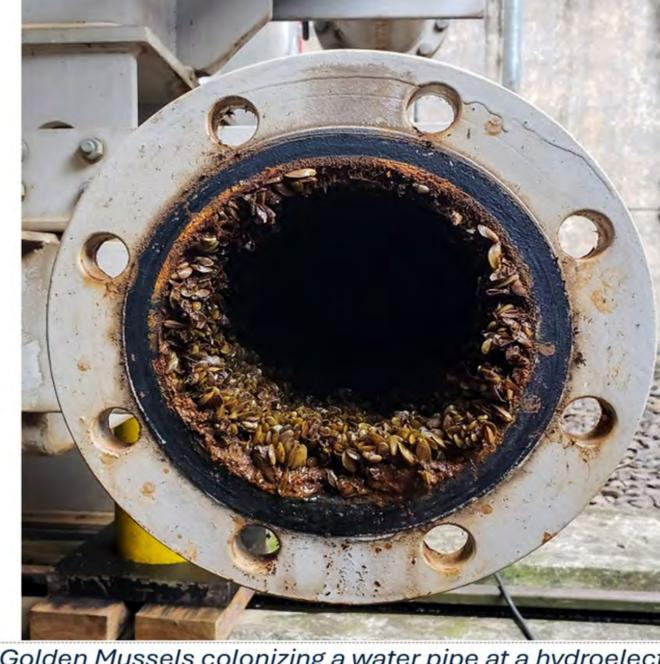
Golden Mussels colonizing a water pipe at a hydroelect plant in Brazil (Mountinho, 2021).
