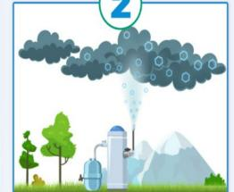
Silver iodide particles mixed with acetone are vaporized and released into the atmosphere using ground based seeding systems. Silver iodide particles rise into cold, high-altitude air; moisture in the air condenses to form ice crystals on the particles. By freezing of droplets and deposition of vapor, ice crystals form and grow progressively larger, forming snowflakes large enough to precipitate to the ground.
