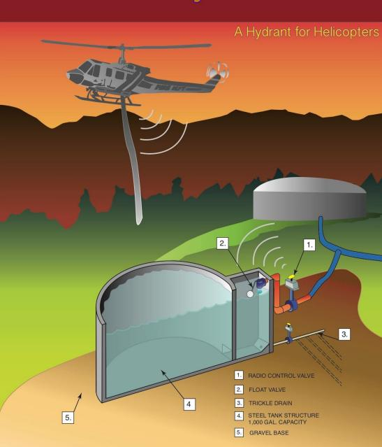
The Heli-Hydrant system allows for rapid aerial response times to fight fires
