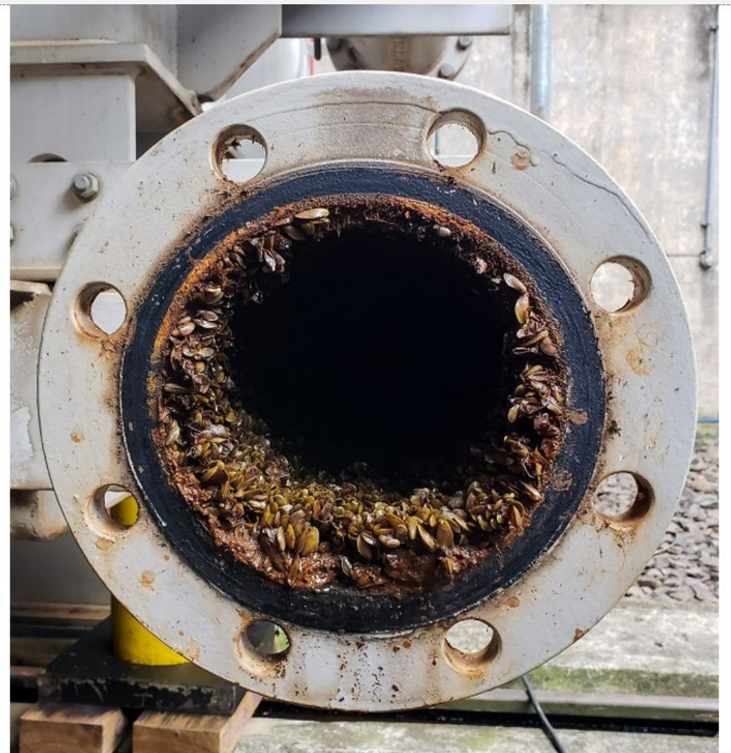
Golden Mussels colonizing a water pipe at a hydroelectric plant in Brazil ( Mountinho, 2021 ).
