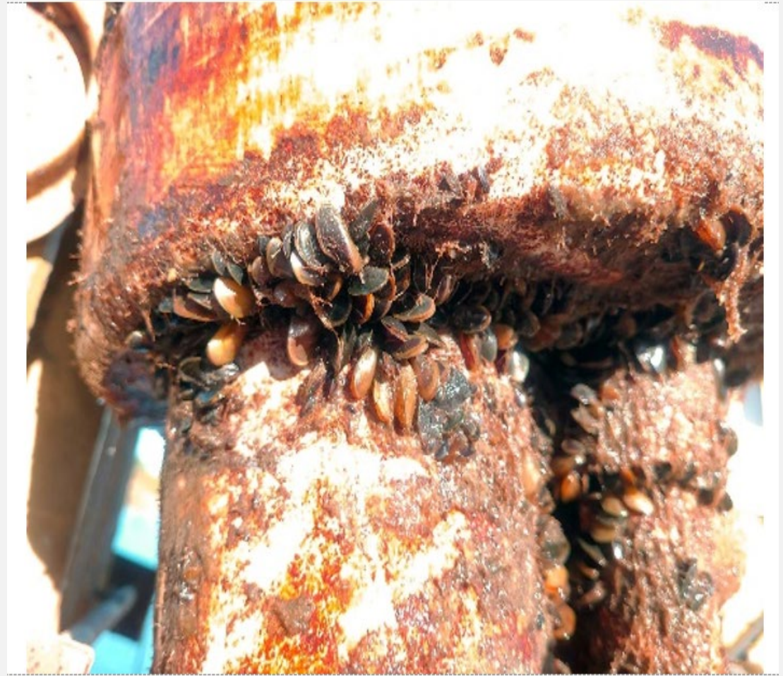
Golden mussels colonizing the exterior housing of water quality equipment at Rough and Ready Island in October 2024. Photo: Jay Aldrich (DWR)
