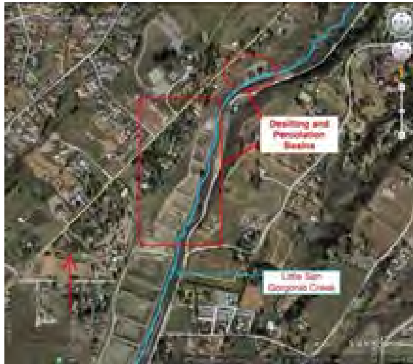
Figure 6-9– Desilting and Recharge Basins at the Mouth of Little San Gorgonio Creek (Edgar Canyon)
