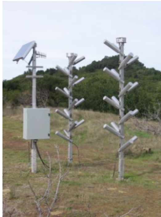
Automated High Output Generating Stations (AHOGS)
