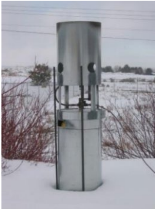
Cloud Nuclei Generators (CNGs)
