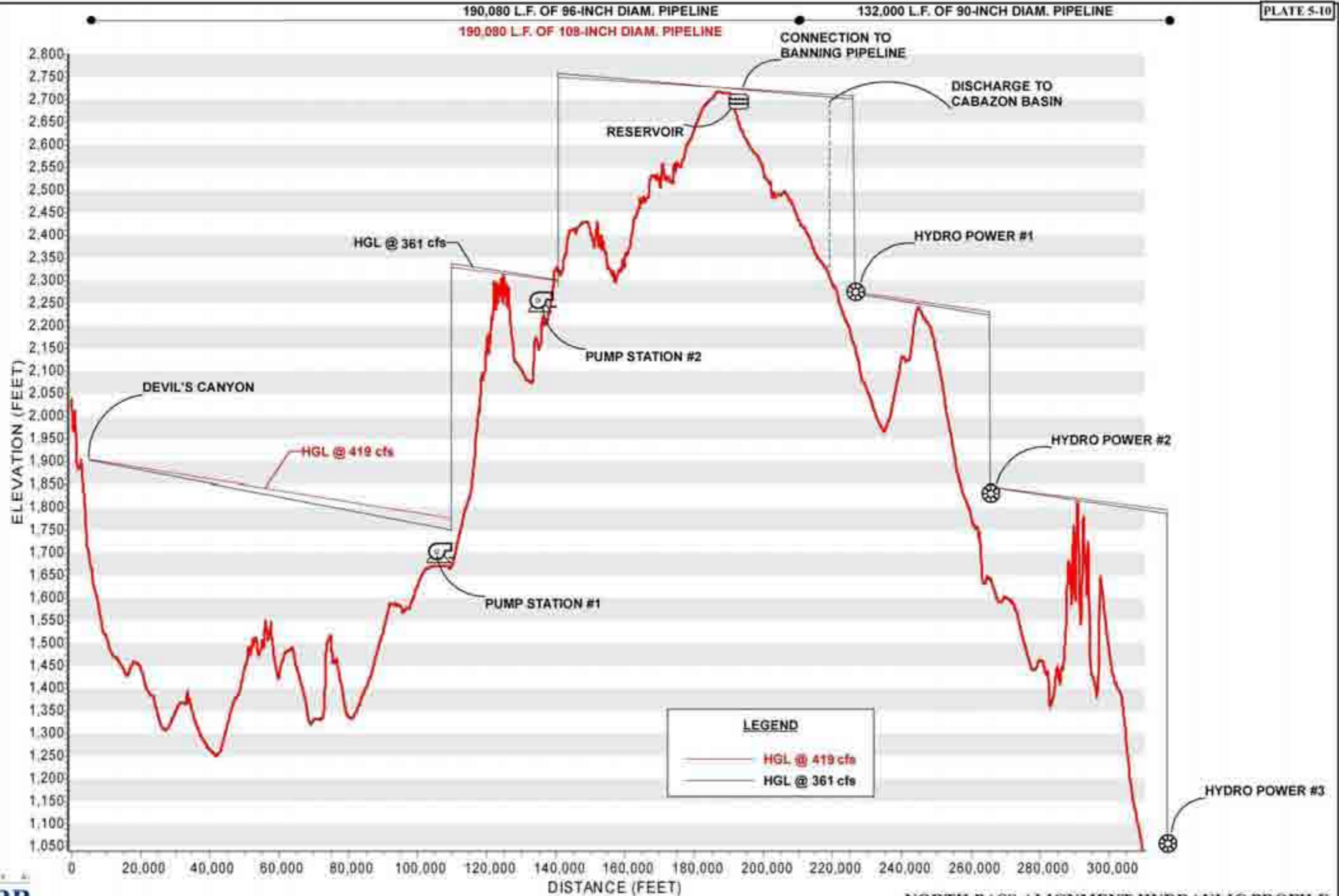
NORTH PASS ALIGNMENT HYDRAULIC PROFILE 63% Reliability
