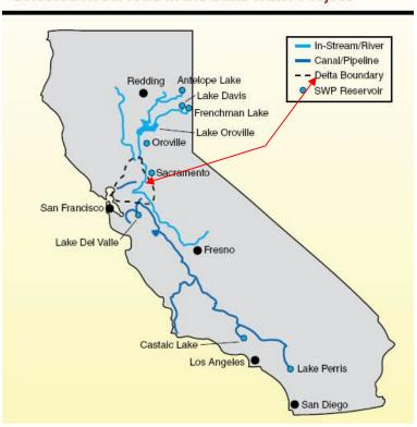
The SWP captures water originating from the Sierra-Nevada Mountains and transports it to 29 State Water Contractors throughout the state. This water would normally flow from the mountains, to various rivers, through the San Joaquin Delta and ultimately be lost to the Pacific Ocean via the San Francisco Bay.
