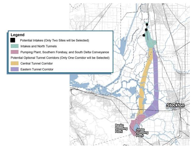
The DCP will consist of two intakes along the northern portion of the Delta, adjacent to the Sacramento River, and approximately 42 miles of tunnel. Two potential routes have been proposed. When completed, the project will have a maximum capacity of roughly
