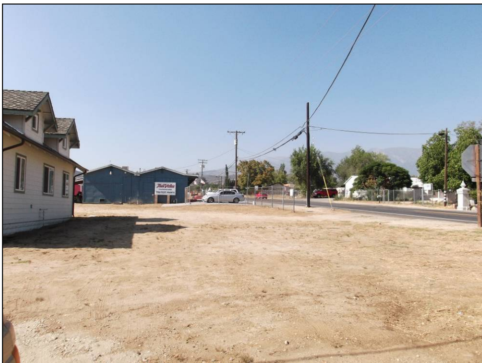
View west from the corner of Beaumont and Vineland showing typical soils near roadways. It is assumed these soils are disturbed to a point at least 2 feet below grade by previous road works and infrastructure impacts.
